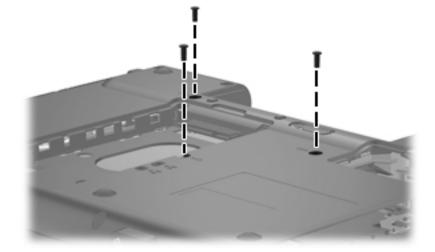
Where used: 3 screws that secure the keyboard to the computer
